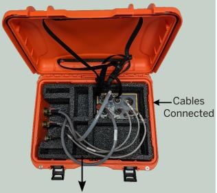
» If using internal power do not connect external power cable to case.
